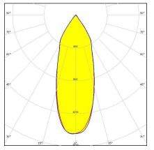
Dimensions: 119.5 mm x 119.5 mm Height: 74.50 mm ~45° wide beam compatible with BJB connectors
