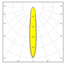
Dimensions: 119.5 mm x 119.5 mm Height: 74.27 mm ~30° medium beam
