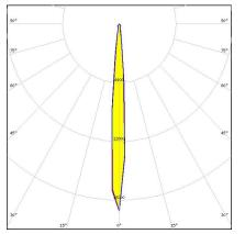
Dimensions: 119.5 mm x 119.5 mm Height: 74.50 mm ~10° spot beam compatible with BJB connectors
