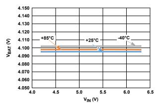
FIGURE 5. NO LOAD VOLTAGE vs TEMPERATURE
