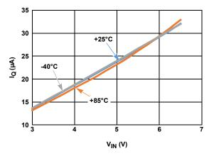
FIGURE 15. INPUT QUIESCENT CURRENT vs INPUT VOLTAGE, SHUTDOWN
