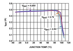
FIGURE 8. CHARGE CURRENT vs JUNCTION TEMPERATURE, **R**IREF = 158k
