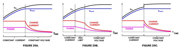
FIGURE 29. THE OPERATING CURVES WITH THREE DIFFERENT CURRENT LIMITED POWER SUPPLIES
