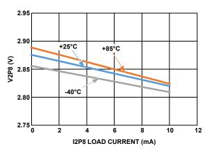
FIGURE 13. V2P8 OUTPUT vs LOAD CURRENT
