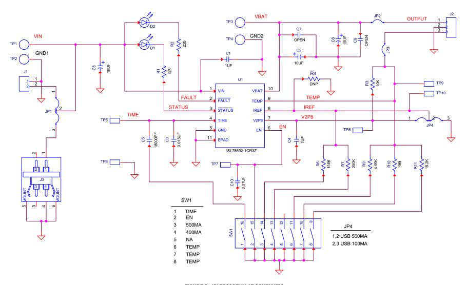
FIGURE 3. ISL78692EVAL1Z SCHEMATIC
