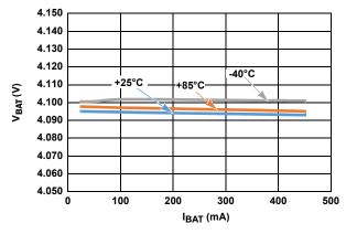
FIGURE 4. VOLTAGE REGULATION vs CHARGE CURRENT
