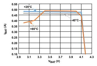
FIGURE 6. CHARGE CURRENT vs OUTPUT VOLTAGE, RIREF = 158k
