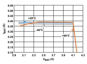
FIGURE 7. CHARGE CURRENT vs OUTPUT VOLTAGE, RIREF = 200k
