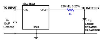
FIGURE 25. INSERTING R<sub>1</sub> TO IMPROVE THE STABILITY OF APPLICATIONS WITH LARGE CERAMIC CAPACITOR USED AT THE OUTPUT
