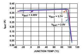
FIGURE 9. CHARGE CURRENT vs JUNCTION TEMPERATURE, **R**IREF = 200k
