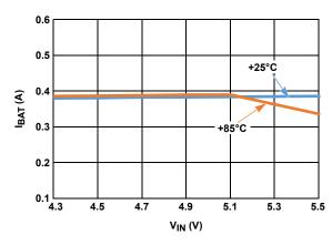
FIGURE 11. CHARGE CURRENT vs INPUT VOLTAGE,  $V_{BAT} = 3V$ ,  $R_{IREF} = 200k$
