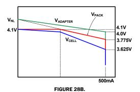
FIGURE 28. THE I-V CHARACTERISTICS OF THE CHARGER WITH DIFFERENT CURRENT LIMITED POWER SUPPLIES
