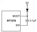
Figure 2. External Bootstrap Diode
