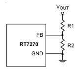
Figure 1. Output Voltage Setting
