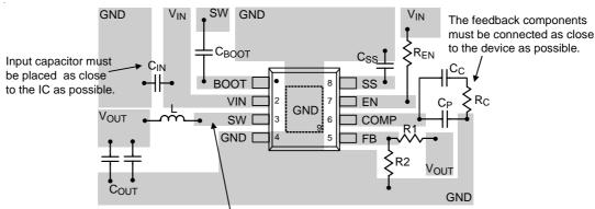
SW node is with high frequency voltage swing and should be kept at small area. Keep analog components away from the SW node to prevent stray capacitive noise pick-up
