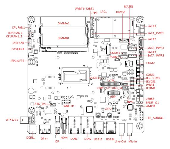
Figure 1.1 Jumper and Connector Location
