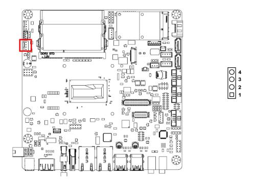
System fan can support Voltage mode and PWN mode by jumper JSYSFAN1.(default is voltage mode).
