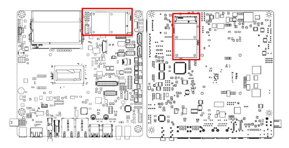
The AIMB-231 provides 1 Full size Mini PCI express slot (Co-lay mSATA & SIM card holder) and 1 Half size Mini PCI express slot.
