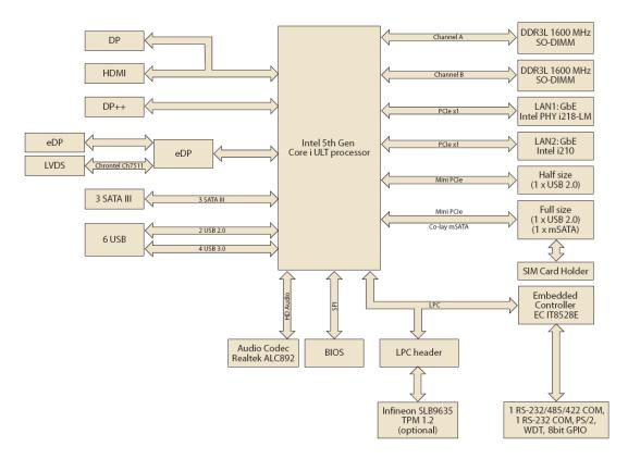
Figure 1.2 AIMB-231 Board Diagram
