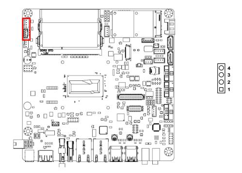
CPU fan can support Voltage mode and PWN mode by jumper JCPUFAN1.(default is voltage mode)
