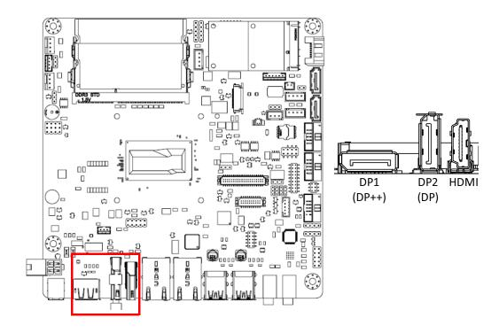
The AIMB-231 includes DP/HDMI and DP++ interface that can drive conventional DP/HDMI and DP++ displays. DP and HDMI only one can be used at same time. default setting is at HDMI.
