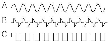
Example A is an undistorted sinewave and the IMH will indicate TRUE RMS. With the complex waveforms shown in examples B and C, the meter will indicate average value.
