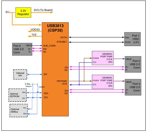
FIGURE 2-3: EVB-USB3813 BLOCK DIAGRAM
