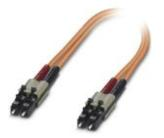
Assembled FO cable, zip cord cable, multi-mode fiberglass 62.5/125 µm, OM1, connector: LC duplex/LC duplex, degree of protection: IP20, for installation in cable ducts or control cabinets
