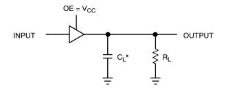
\*Includes all probe and jig capacitance. A 1-MHz square input wave is recommended for propagation delay tests.
