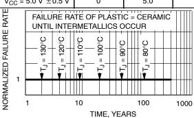
Figure 3. Failure Rate versus Time Junction Temperature
