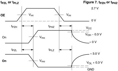
Figure 8. AC Output Enable and Disable Waveform
