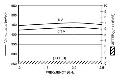
Figure 3.  $F_{max}/Jitter @ 25^{\circ}C$
