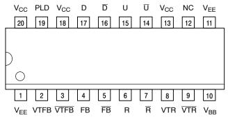
Warning: All  $V_{CC}$  and  $V_{EE}$  pins must be externally connected to Power Supply to guarantee proper operation.
