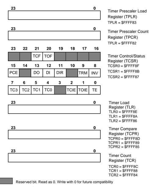
Figure 9-20. Timer Module Programmer's Model
