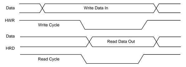
In dual-strobe mode, separate HRD and HWR signals specify the access as a read or write access, respectively.
