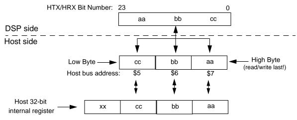
Figure 6-4. HI08 Read and Write Operations in Little Endian Mode
