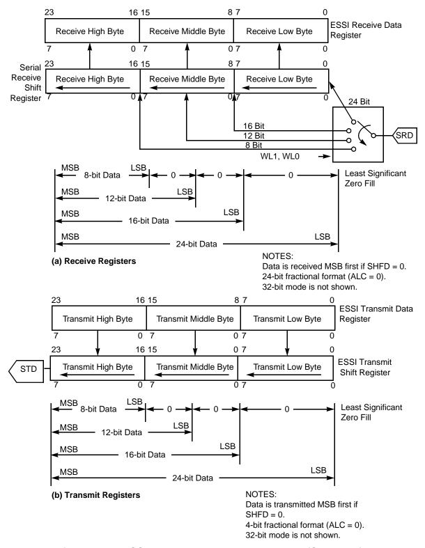
Figure 7-12. ESSI Data Path Programming Model (SHFD = 0)
