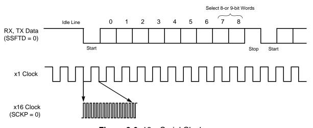
Figure 8-6. 16 x Serial Clock
