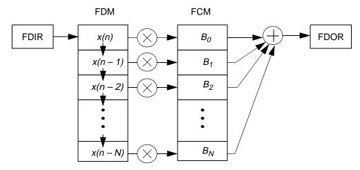
Figure 10-4. FIR Filter Type Processing
