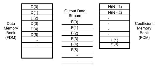
Figure 10-6. Real FIR Filter Data Stream
