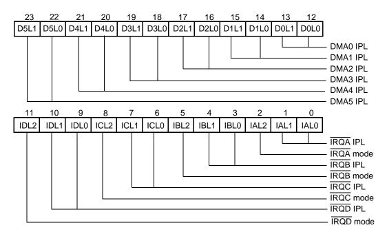
Figure 4-3. Interrupt Priority Register-Core (IPRC) (X:\$FFFFFF)
