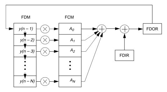
Figure 10-5. IIR Filter Type Processing
