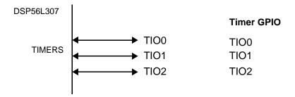
Figure 5-6. Triple Timer Signals
