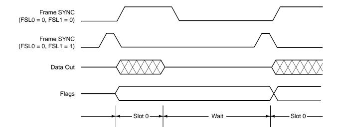
Figure 7-9. Normal Mode, External Frame Sync (8 Bit, 1 Word in Frame)
