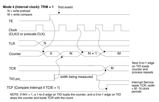
**Figure 9-11.** Pulse Width Measurement Mode, TRM = 1
