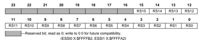
Figure 7-16. ESSI Receive Slot Mask Register A (RSMA)
