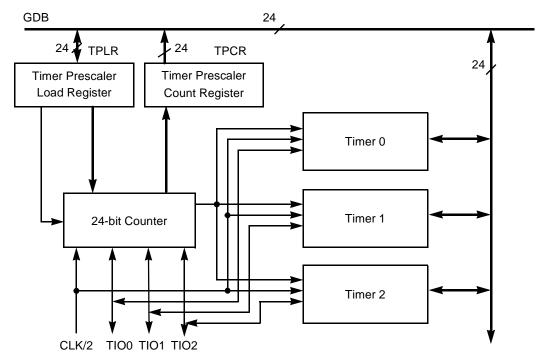
Figure 9-1. Triple Timer Module Block Diagram
