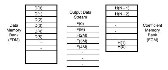
Figure 10-7. Real FIR Filter Data Stream With Decimation by M
