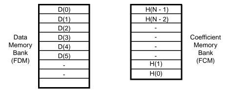
Figure 10-2. Storage of Filter Coefficients
