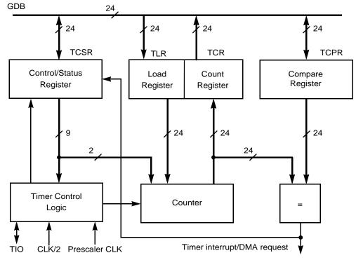
Figure 9-2. Timer Module Block Diagram
