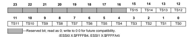
Figure 7-14. ESSI Transmit Slot Mask Register A (TSMA)
