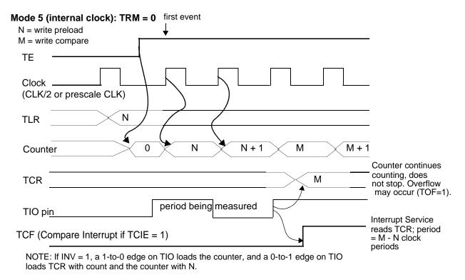
**Figure 9-14.** Period Measurement Mode, TRM = 0
