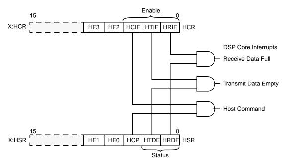
Figure 6-2. HI08 Core Interrupt Operation
