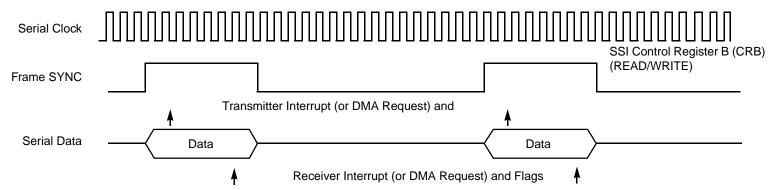
NOTE: Interrupts occur and data is transferred once per frame sync.
