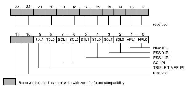
Figure 4-4. Interrupt Priority Register-Peripherals (IPRP) (X:\$FFFFFE)
