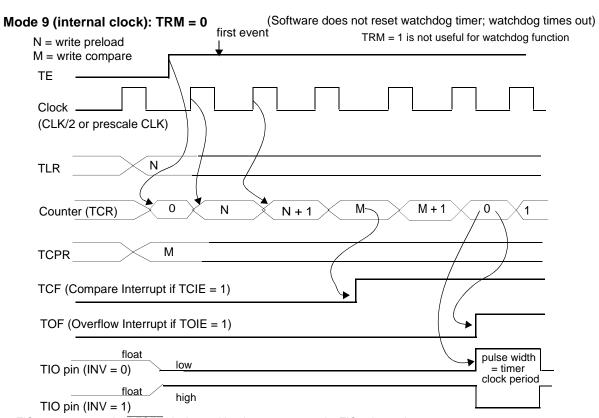
TIO can connect to the  $\overline{\text{RESET}}$  pin, internal hardware preserves the TIO value and direction for an additional 2.5 clocks to ensure a reset of valid length.
