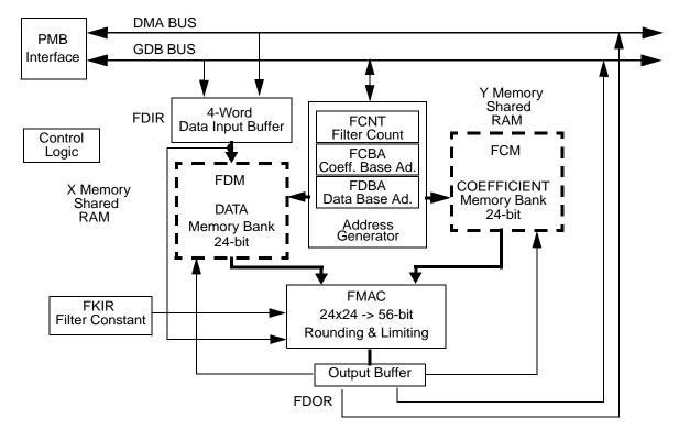
Figure 10-1. EFCOP Block Diagram
