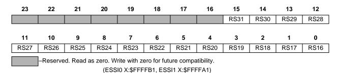
Figure 7-17. ESSI Receive Slot Mask Register B (RSMB)
