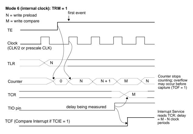
NOTE: If INV = 1, a 1-to-0 edge on TIO loads TCR with count and stops the counter.
