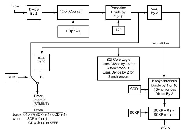
Figure 8-5. SCI Baud Rate Generator
