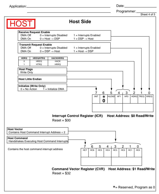
Figure B-13. Interrupt Control and Command Vector Registers
