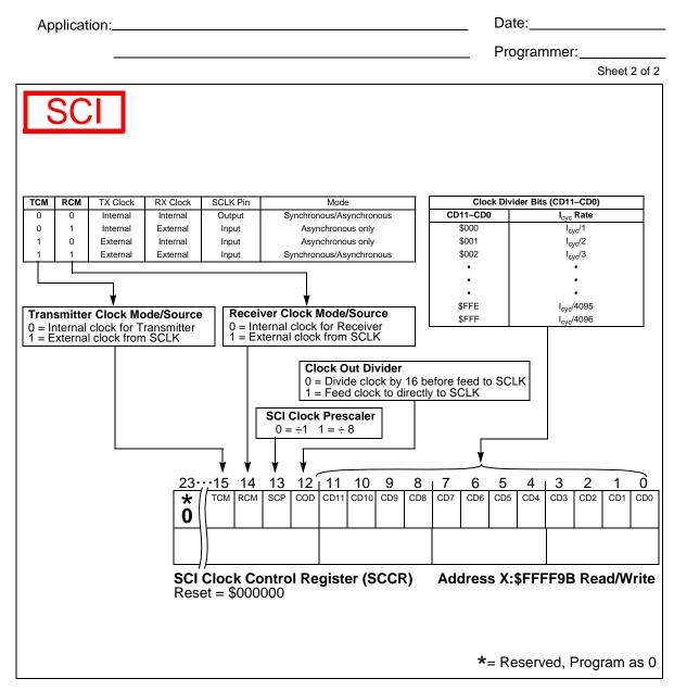
Figure B-19. SCI Clock Control Registers (SCCR)
