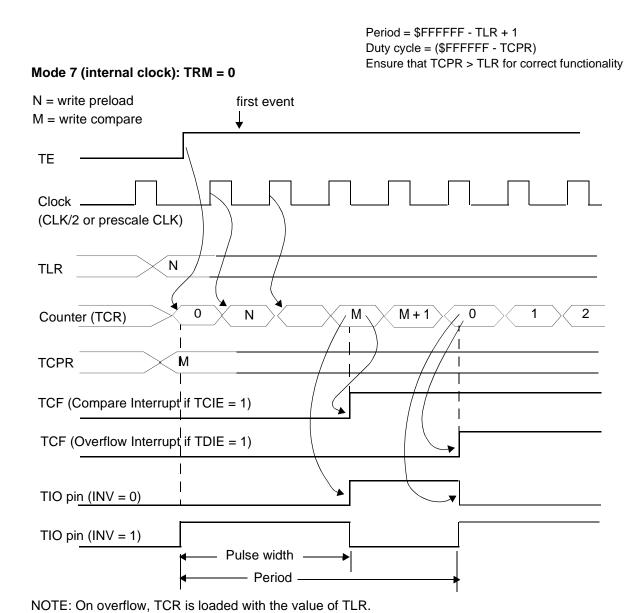
Figure 9-17. Pulse Width Modulation Toggle Mode, TRM = 0
