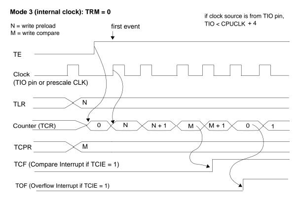
NOTE: If INV = 1, counter is clocked on 1-to-0 clock transitions, instead of 0-to-1 transitions.
