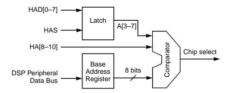
Figure 6-11. Self Chip-Select Logic
