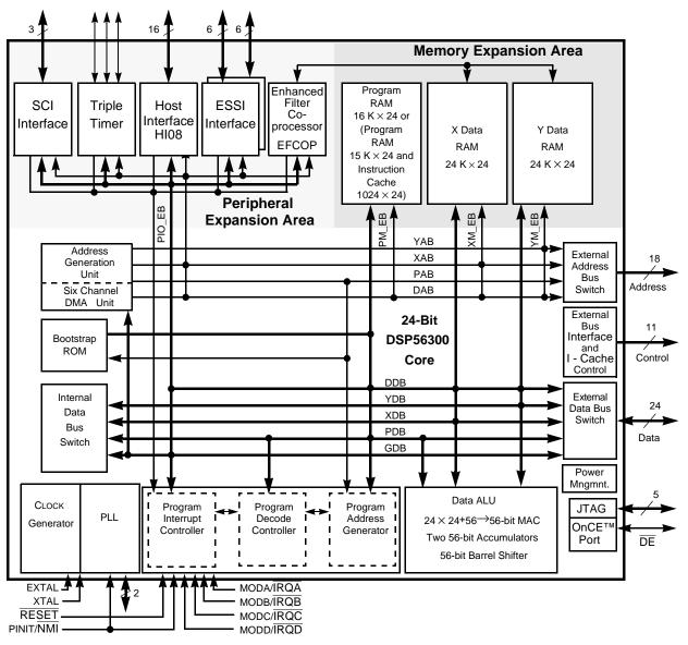
Figure 1-1. DSP56L307 Block Diagram
