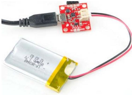
You can also use your own 5V supply and charge over the charge pins labeled '5V' and 'GND'.
