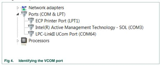
If the J-Link firmware image has been programmed into the Debug Probe and DFU boot mode is not being used, then a VCOM device called Jlink CDC UART port will appear instead of the LPC-LinkII UCom port.
