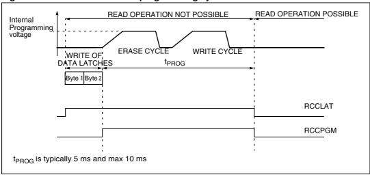
Figure 8. RC user calibration programming cycle
