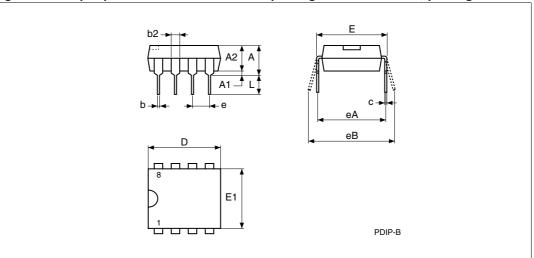
Figure 45. 8-pin plastic dual in-line outline package - 300-mil width, package outline
