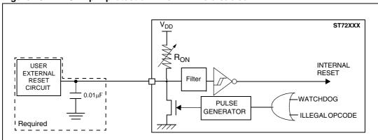
Figure 40. RESET pin protection when LVD is disabled
