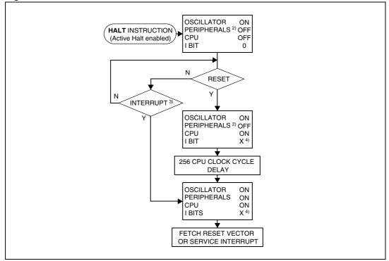
Figure 21. Active-halt mode flowchart
