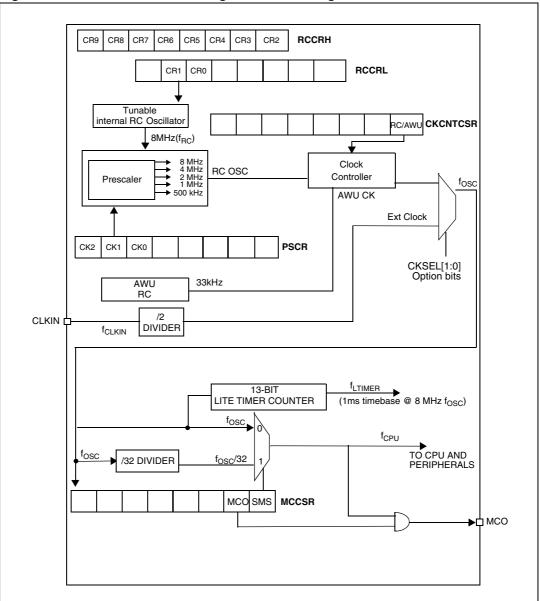
Figure 10. ST7FOXU0 clock management block diagram
