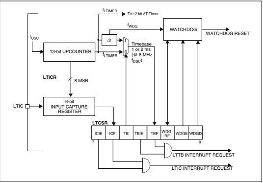
Figure 29. Lite timer block diagram
