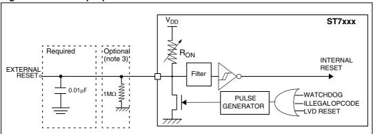
Figure 39. RESET pin protection when LVD is enabled
