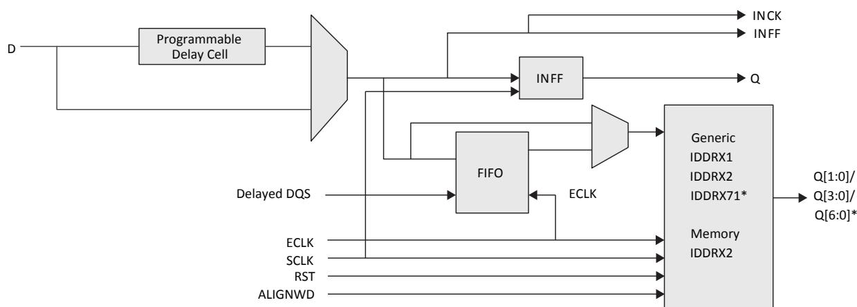
\*For 7:1 LVDS interface only. It is required to use PIO pair pins (PIOA/B or PIOC/D).
