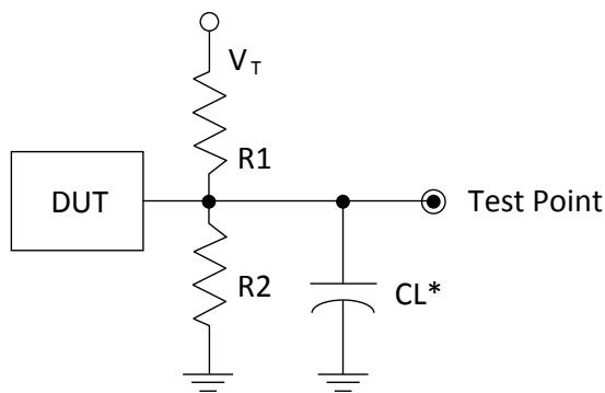
\*CL Includes Test Fixture and Probe Capacitance
