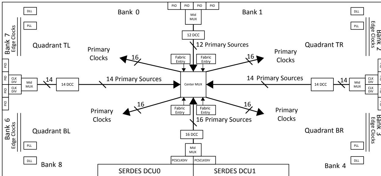
Figure 2.6. LFE5UM/LFE5UM5G-85 Clocking
