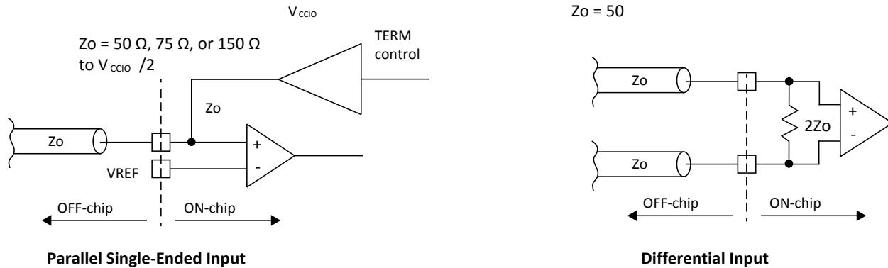
Figure 2.26. On-Chip Termination
