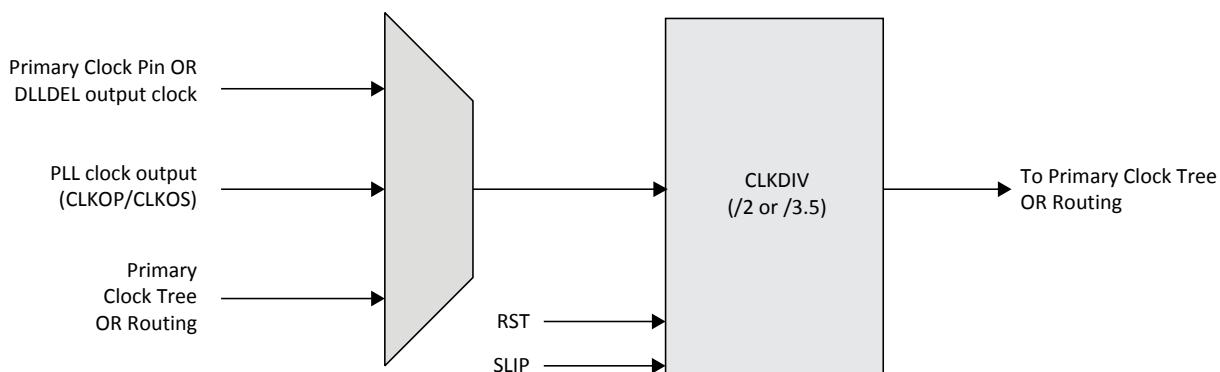
**Figure 2.9. ECP5/ECP5-5G Clock Divider Sources**
