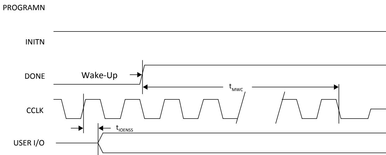
**Figure 3.21. Wake-Up Timing**
