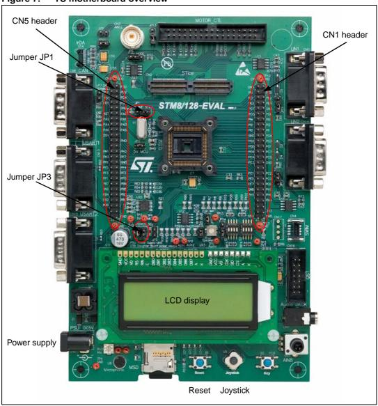
When using the STM8S TS daughterboard assembled with the STM8/128-EVAL (mother) board, the following settings must be implemented:
