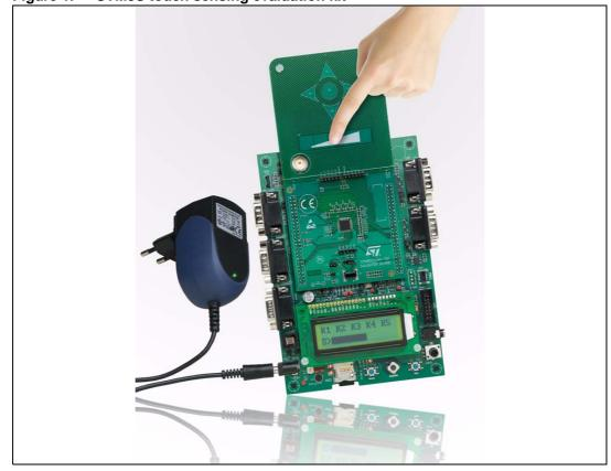
Figure 1. STM8S touch sensing evaluation kit
