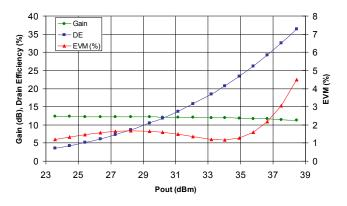
Figure 7 - Gain, Efficiency, EVM at 2500MHz
