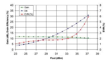
Figure 9 - Gain, Efficiency, EVM at 2700MHz
