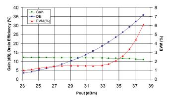
Figure 8 - Gain, Efficiency, EVM at 2600MHz
