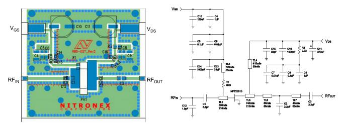
Figure 6 - APP-NPT25015-25 Demonstration Board and Schematic
