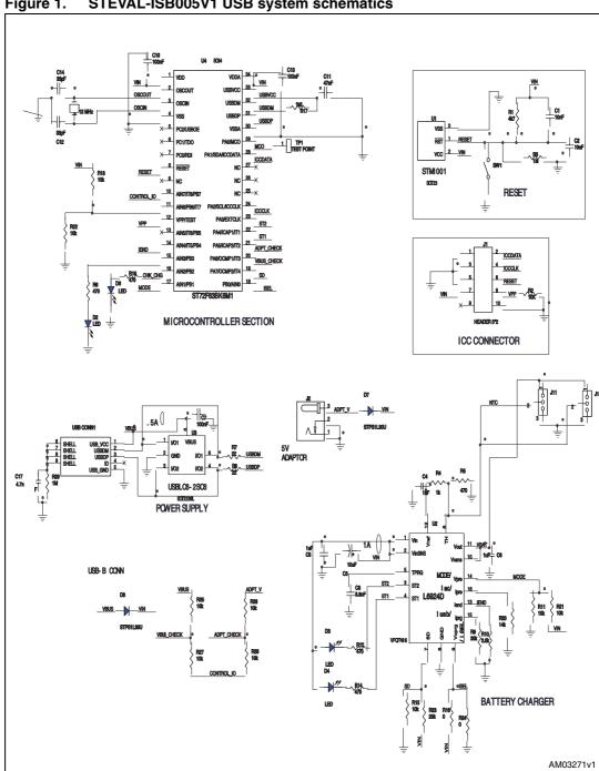
Figure 1. STEVAL-ISB005V1 USB system schematics
